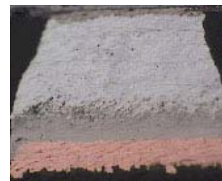
Fig. 12: FC Solder bump after assembly
